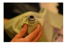
Step 4: Pull the knob out of the boot until the O-ring will not allow you to pull any further. Re-install shift boot/knob assembly. Set desired height of the shift knob and tighten the set screws at the base of the knob.
