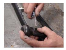
Step 3: Turn the boot inside out and insert the Rennline knob until the base of the knob is even with the base of the boot. Install rubber O-ring over the boot and align with the grove in the knob.
