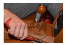
Step 2: For cars with integrated boot/knob, use a razor blade to cut the factory boot all the way around base of the factory knob leaving boot as long as possible. Remove factory knob from the boot. For cars without integrated boot/knob, skip to step 3.
